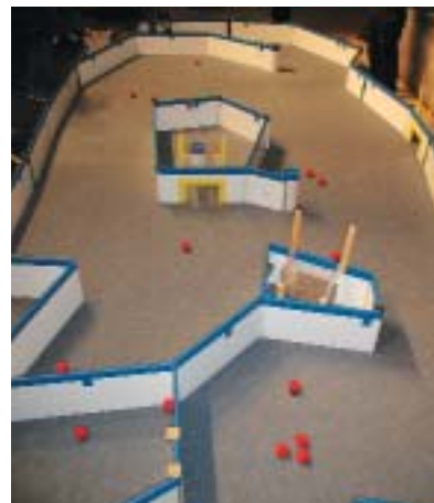
So that programming an entire vision system within one month can be a feasible undertaking, objects in the playing field are kept to a basic set of colors: white, blue, yellow, green, black, red, and light blue.
