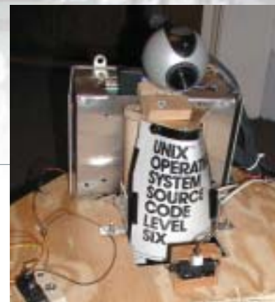
In 2006, Gautham Arumilli, Andrew Muth, Justin Rigling and Matthew Spencer built a robot that stored balls in a column so that it could sense how many balls it had.
