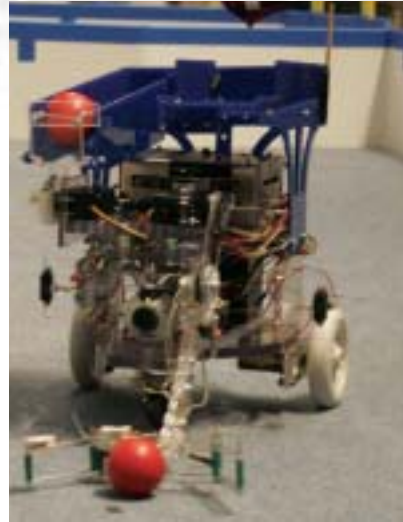
In 2005, Jason Furtado, Nestor Hernandez, Josiah Rosmarin, and Derik Thomann were able to successfully integrate into their robot's design an articulated arm that lifted balls into an overhead bin.
